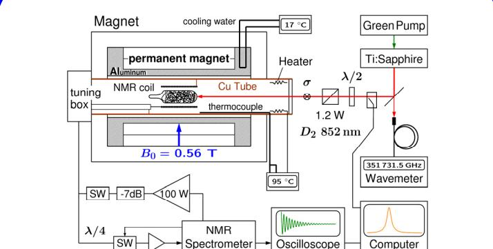
CW pumping light was linearly polarized and routed into a permanent magnet. Cylindrical cell was filled with glass wool. Free-induction decay of Cs salts was detected by a solenoid coil. NMR Trace was Fourier transform of the transient signal.
