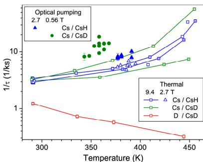
The decay rate of optically enhanced signals ( $\bullet$ ) was larger than the thermal ones. The decay rate increases for Cs ( $\square$  and  $\triangle$ ) and decreases for D ( $\square$ ) as heating. The temperature dependence is super-exponential and it indicates that the hydride is dissociative.
