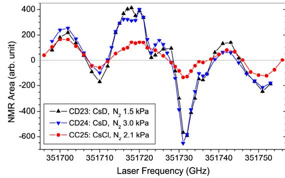
NMR enhancement was measured by scanning laser frequency for CsD salt ( $\blacktriangle$  and  $\blacktriangledown$ ) and CsCl salt ( $\bullet$ ). The identical spectral shape indicates that the nuclear spin polarization of Cs atoms were injected into the salts.
