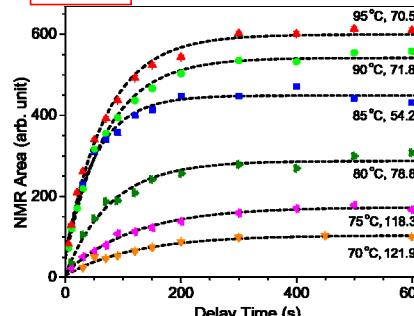
Saturation recovery of spin polarization of CsD at the respective temperatures. See figure on "Curing of Alkali Salt Cell" for the steady-state amplitude. The optimum amplitude was obtained at 95 °C. See figure on "Decay Rate" for the time constant of recovering.
