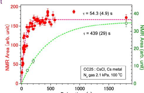
Spin buildup and decay behaviors for CsCl at 100 °C. The bottom inset shows that the saturation RF pulses initialized the spin polarization at  $t=0$ .
