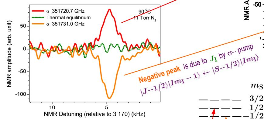
NMR enhancement of CsH salt by  $D_2$  pumping with  $\sigma$  light at 0.56 T. Thermal signal was too small to be detected. Each spectrum was a Fourier transform after averaging 70-shots of FIDs. RF pulses were applied with a tipping angle of  $\pi/3$  every 100 s. CsH crystallites and the excess Cs metal were contained in CH13 cell filled with  $\text{N}_2$  gas of 11 Torr.
