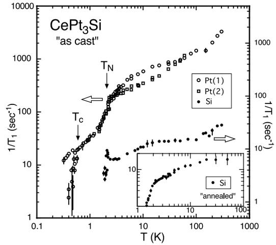
Fig. 2. Temperature dependence of spin-lattice relaxation rate ( $1/T_1$ ) of Pt(1) site, Pt(2) site and Si site in “as cast” sample. Inset is that of Si site in “annealed” sample.
