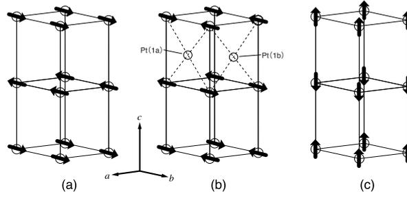
**FIGURE 3.** Magnetic structures of  $\text{CePt}_3\text{Si}$ . Arrows indicate the direction of the magnetic moment at Ce site. (a) A magnetic structure proposed by Metoki *et al.* (b) One of the magnetic structures to make the  $c$ -axis component with the moment lying in the basal  $c$ -plane. (see text) (c) A possible magnetic structure with the magnetic moment along the  $c$ -axis.
