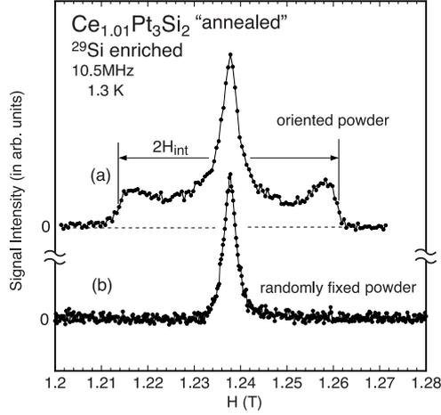
**FIGURE 1.** NMR spectra of  $^{29}\text{Si}$  nuclei obtained under different sample condition in “annealed”  $\text{Ce}_{1.01}\text{Pt}_3\text{Si}_2$  at 1.3 K. (a) A spectrum of the powder sample ( $\mathbf{H} // c$ -axis). The full line width corresponds to the internal field ( $2H_{\text{int}}$ ). (b) A spectrum of the powder sample (non aligned to magnetic field).
