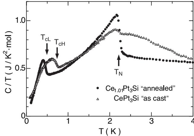
**FIGURE 4.** Temperature dependence of the specific heat in the form of  $C/T$  of  $\text{CePt}_3\text{Si}$ . Closed circles and open triangles show the data of “annealed” sample and “as cast” sample, respectively.  $T_{cL}$  and  $T_{cH}$  mean low  $T_c$  and high  $T_c$ , respectively. (see text)
