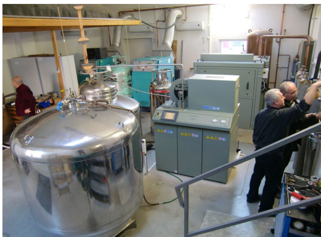
Helium Liquefier Linde Model 1410 in cryogenic centre of Department of Low Temperature Physics, Slovak Academy of Sciences, Kosice, Slovakia.
