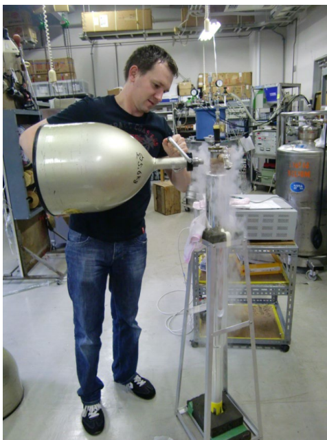
Filling of glass cryostat with liquid nitrogen (Hyogo University, Japan).
