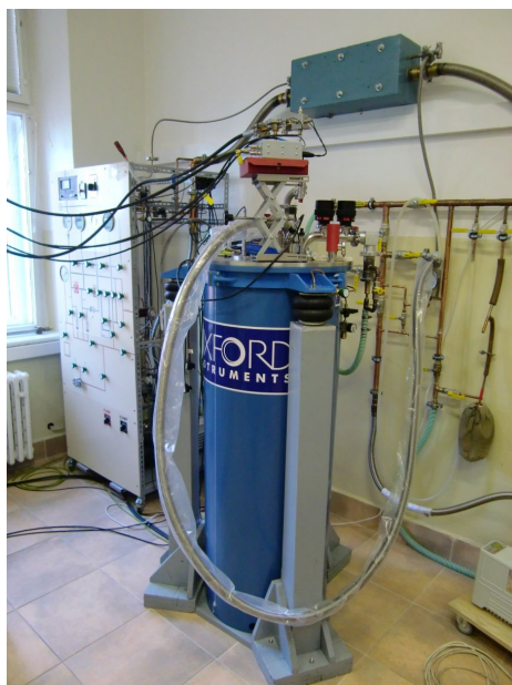
Cryostat in laboratory for high pressure physics. Lowest temperature achieved with mini dilution refrigerator (MINIFRIDGE) is 50 mK
